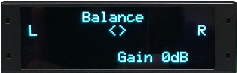
**BALANCE** Channel balance adjustment (right and left)
