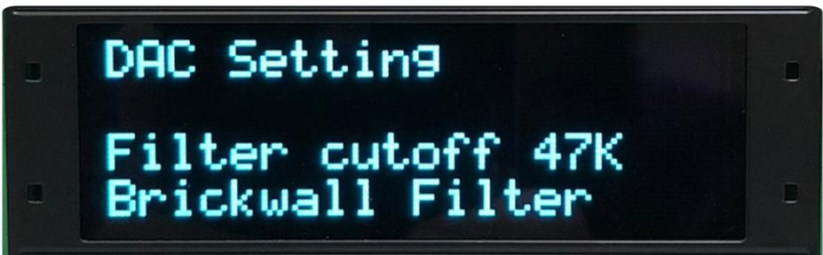
**DAC Setting** D/A filter slope and their roll-off adjustment
