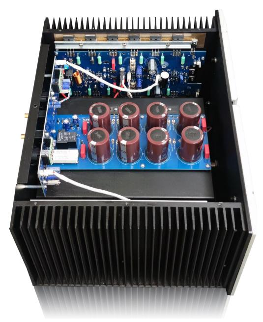
The power transformer, in addition to being shielded, is mounted under an iron cover which further increases its rejection of disturbances. The entire filter bank and the rectifier diodes are instead mounted on a PCB with 70 micron copper without air wiring.
