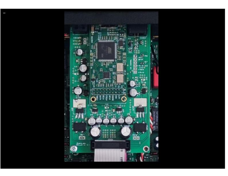
The DAC reads files with conversion up to 384 Khz in PCM and DSD 256 in Dop or DSD 512 natively.
